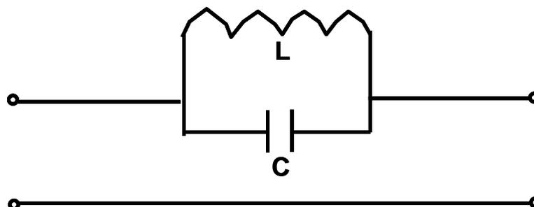
Figure 2. The equivalent circuit of the DGS unit
