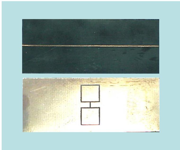
**Figure 4. Fabricated 50  $\Omega$  microstrip line and the DGS unit (The DGS gap length,  $c$  and the distance,  $d$  are 2 mm and 0.1 mm. The DGS dimensions are,  $a= 6$  mm,  $b= 5.8$  mm.)**
