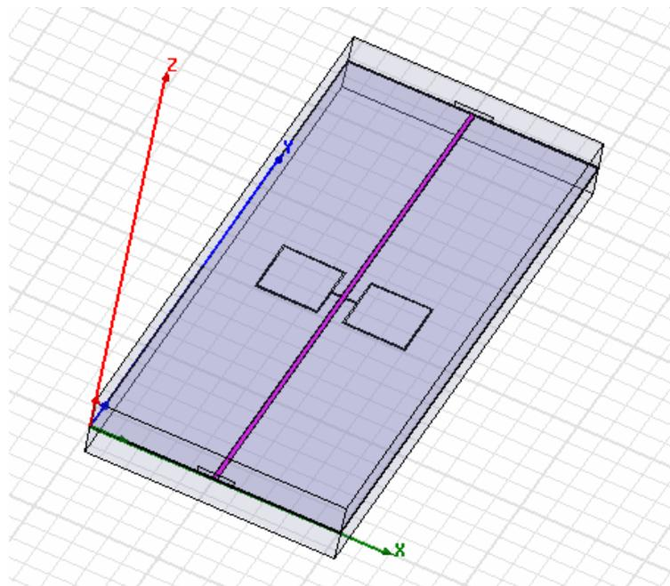
Figure 3. 3-D View of the DGS unit (etched in the conducting ground layer of a microstrip line)
