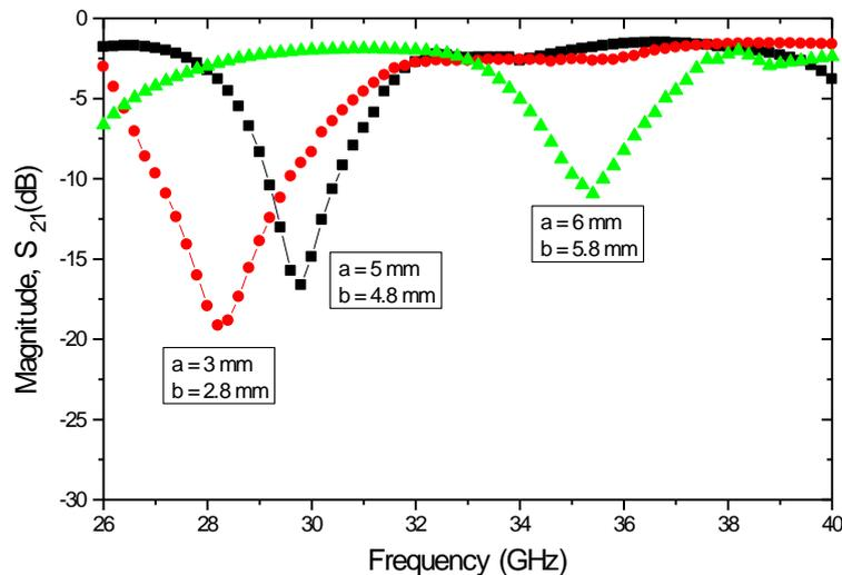
**Figure 6.** Simulated  $S_{21}$  parameters (The DGS gap length,  $c$  and the distance,  $d$  are 2 mm and 0.1 mm, for all cases. DGS dimensions are,  $a=3$  mm,  $b=2.8$  mm;  $a=5$  mm,  $b=4.8$  mm; and  $a=6$  mm,  $b=5.8$  mm.)
