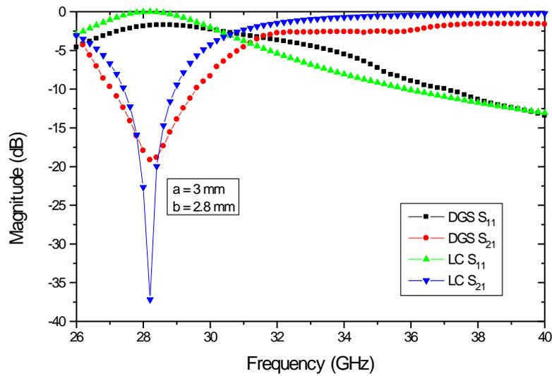
**Figure 5.** Comparison of the simulated S-parameters of the DGS unit and equivalent series-connected parallel LC resonance circuit (The DGS gap length,  $c$  and the distance,  $d$  are 2 mm and 0.1 mm. The DGS dimensions are,  $a=3$  mm,  $b=2.8$  mm.)
