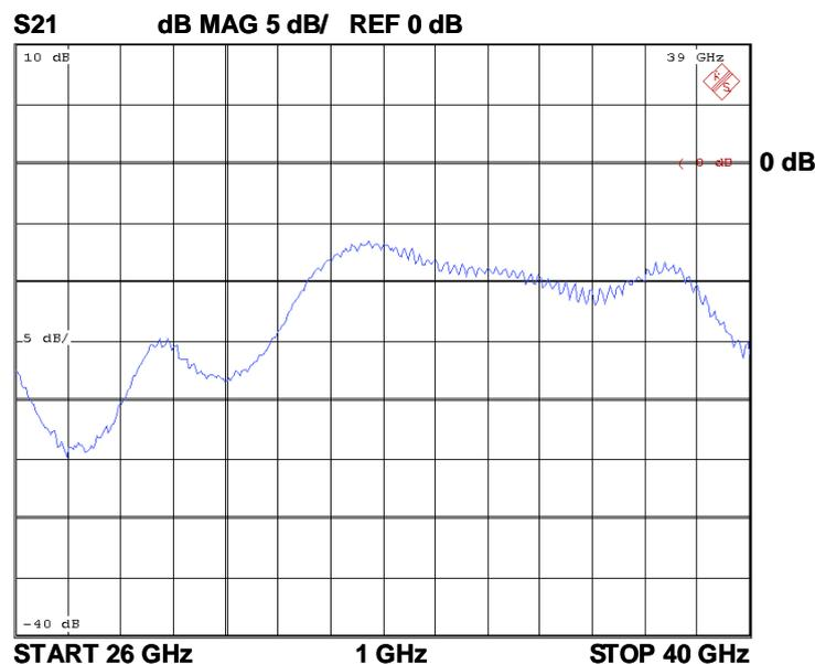
Figure 7. Measured  $S_{21}$  for the DGS unit (The DGS gap length,  $c$  and the distance,  $d$  are  $2\text{ mm}$  and  $0.1\text{ mm}$ . The DGS dimensions are,  $a=3\text{ mm}$ ,  $b=2.8\text{ mm}$ .)
