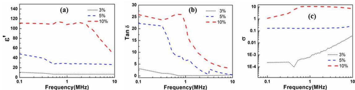
Figure 2. (a), (b), (c)  $\epsilon'$ ,  $\tan \delta$ , and  $\sigma$  as a function of frequency, for different Gr%
