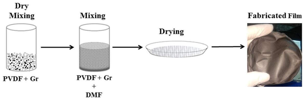
Figure 1. Fabrication process of conducting film
