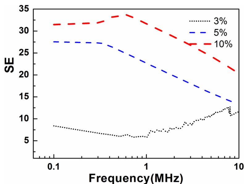
Figure 3. SE as a function of frequency for different Gr wt %
