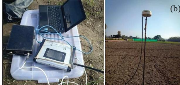
**Figure 1** (a) Setup for receiver. (b) Antenna fixed at 2.16 meter above the ground surface.
