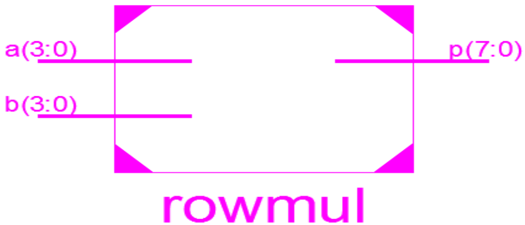
Figure 6. Block diagram of 4*4 row bypassing multiplier
