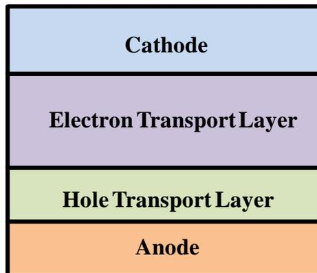
**Figure 2. Structure of bilayer OLED**
