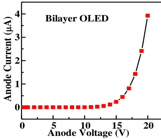
Figure 4. Anode voltage vs. anode current of the bilayer OLED
