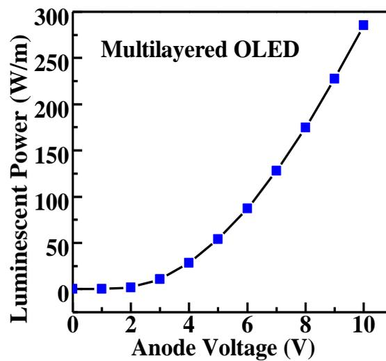
Figure 9. Anode voltage vs. luminescent power of multilayer OLED.
