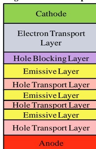
Figure 6. Structure of multilayer OLED
