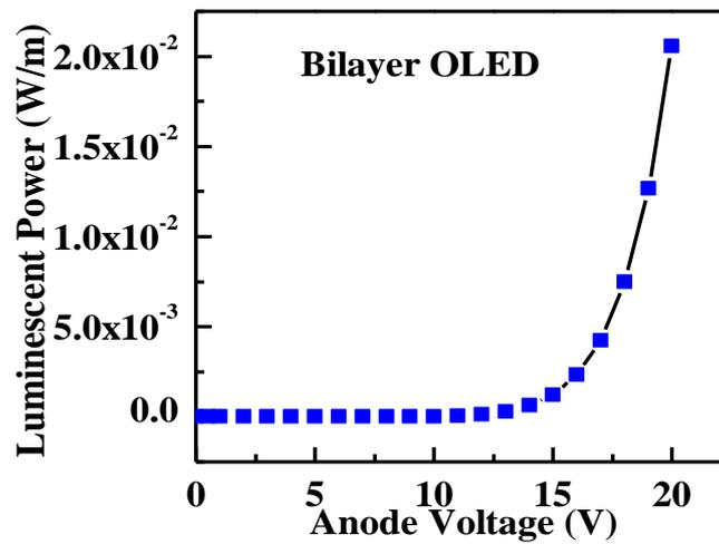
Figure 5. Anode voltage vs. luminescent power of bilayer OLED
