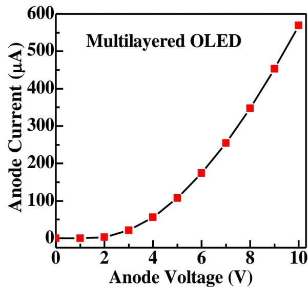
Figure 8. Anode voltage vs. anode current of the multilayer OLED
