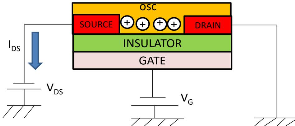
Figure 3.1 Schematic of biased OTFT device
