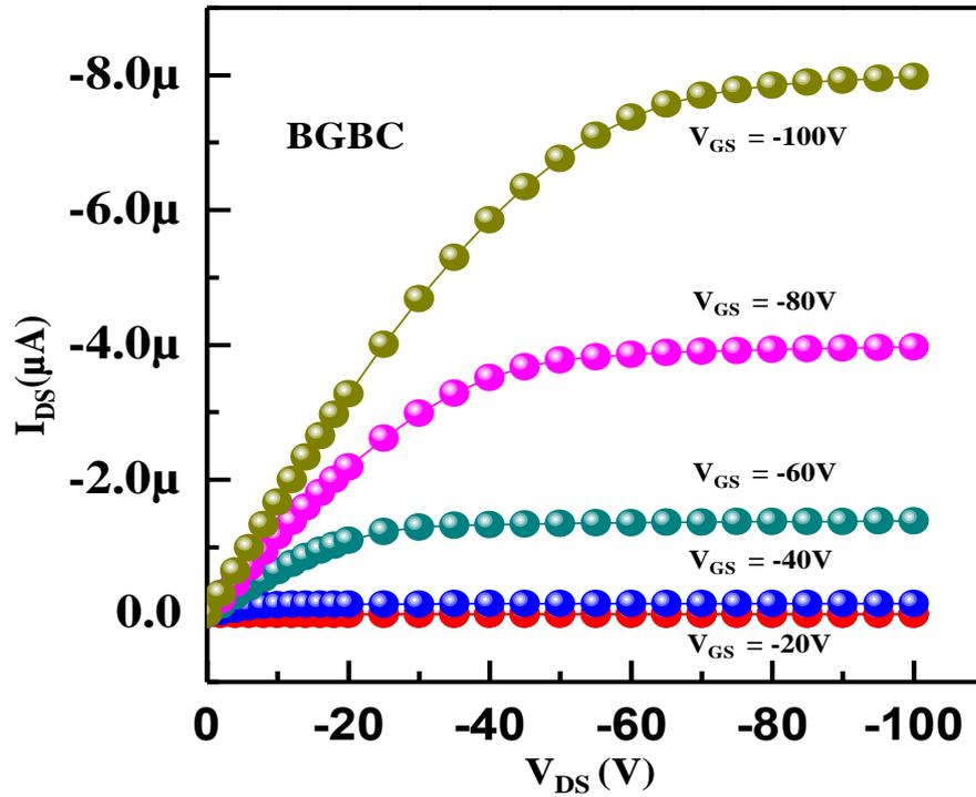
Figure 6.1 Output characteristics of bottom gate bottom contact structure
