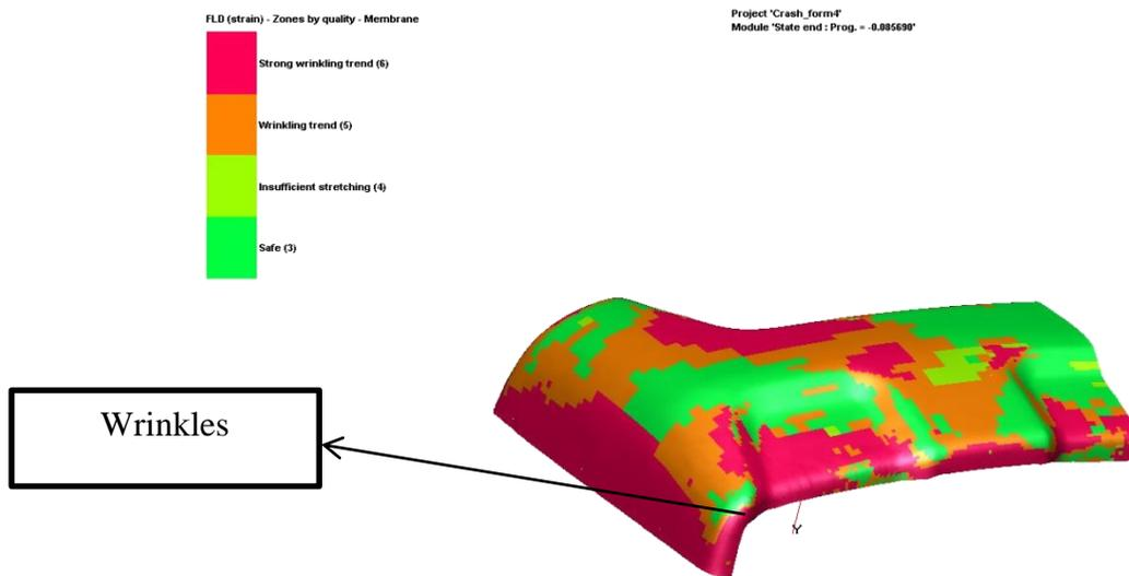
Figure 3. Shows the wrinkles during simulation
