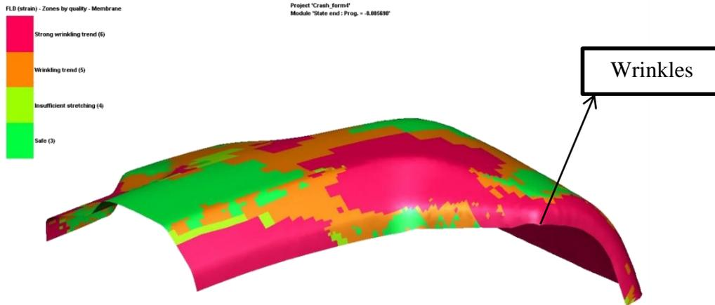
Figure 2. Shows the wrinkles during simulation
