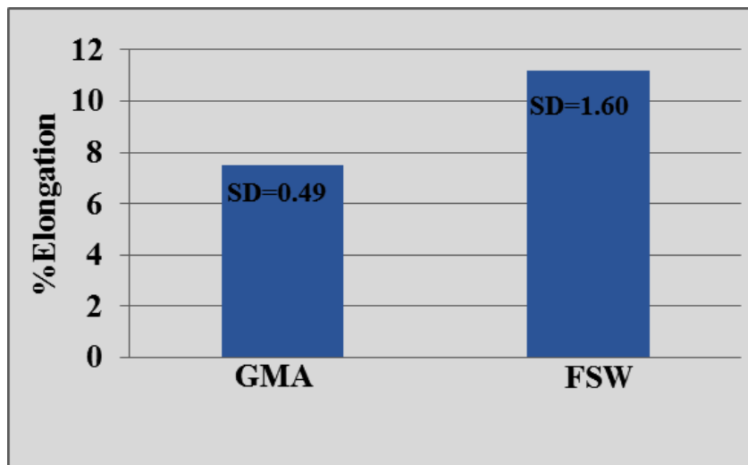
Figure 2. Percentage of elongation of GMA and FSW welded joints
